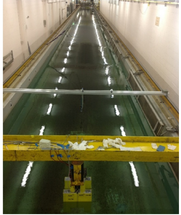
Figure 5: A general view of the AMC towing tank showing the OWC model installed in the tank, looking towards the beach.
