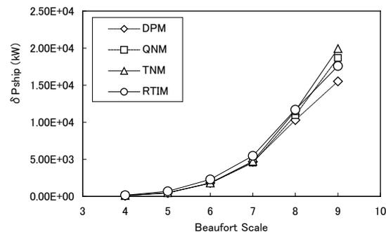
Figure 2: Power increase in irregular waves, VLCC (FULL)
