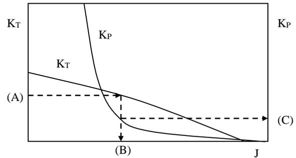
Figure 6: Propeller Open Water Chart (TNM)
