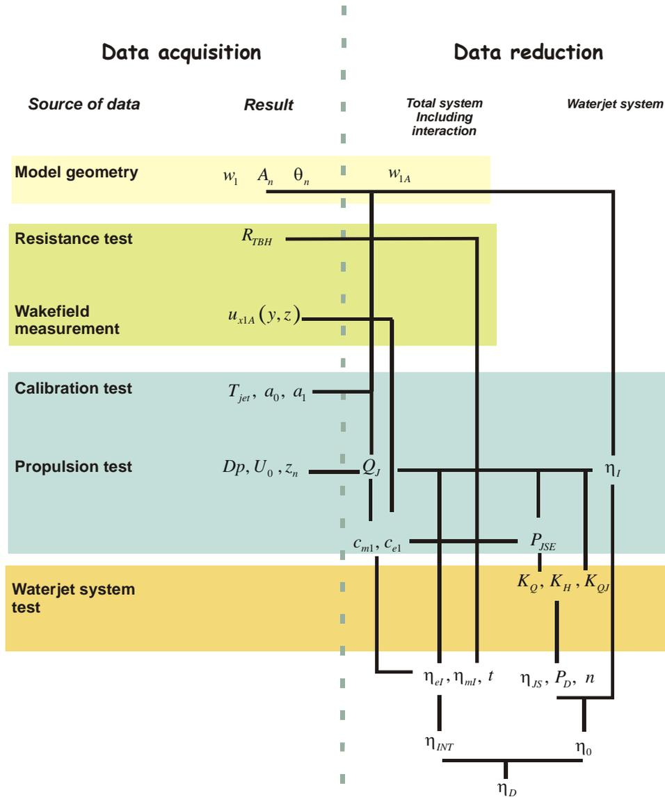
Figure 1 Dataflow in analysis of propulsion test results
