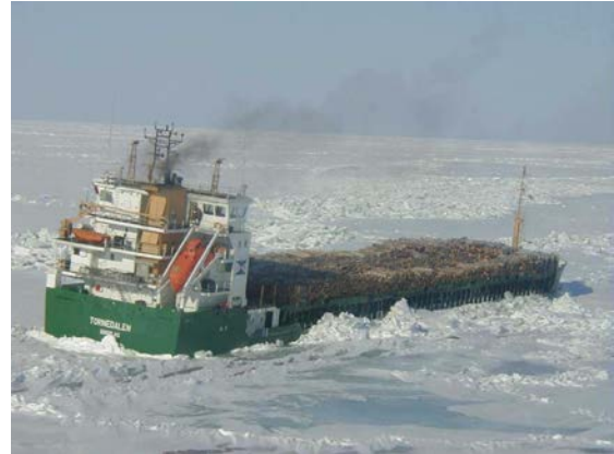
Figure 13: A ship stuck in compressive ice
