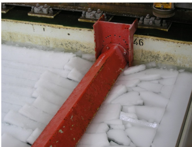
Figure 2: Beam with inclined face breaking the ice downwards
