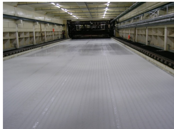
Figure 1: Ice sheet cut free at the sides
