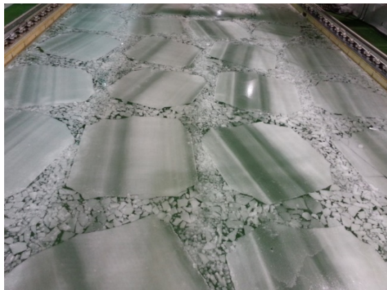
Figure 11: managed ice field in the model basin (60 m long and 12 m wide basin as an example)
