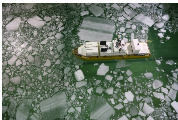
Figure 4: A mixture of floe size in the model basin
