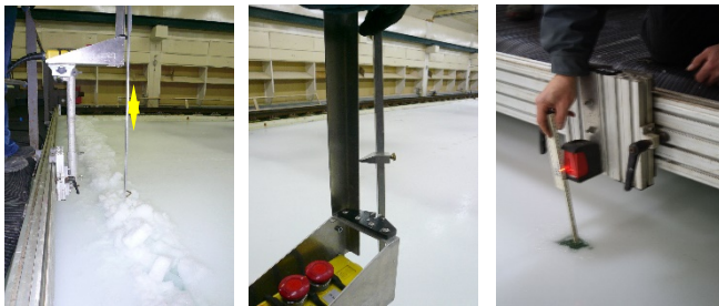
Figure 10 Ridge-profiling device to determine keel depth and sail height
