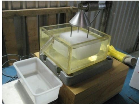
Figure 7: Ex-situ density measurement setup (Option A)
