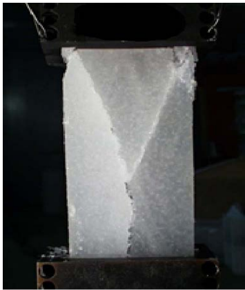
Figure 6: Compressive ex-situ test setup
