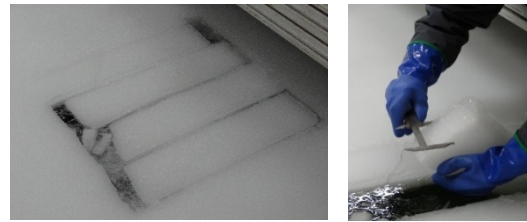
Figure 9: Ice thickness measurements with calliper
