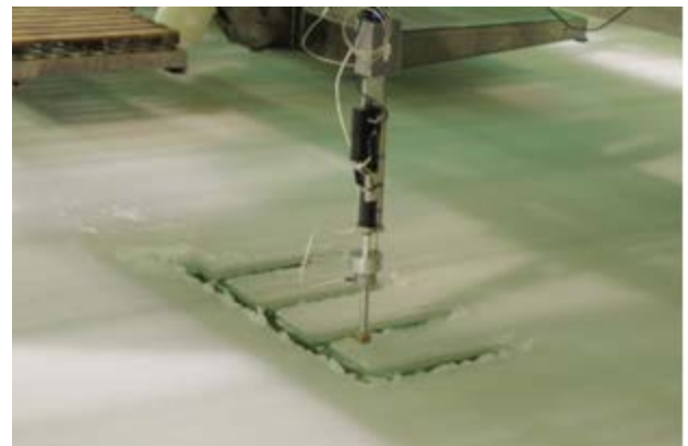
Figure 2: Setup of in-situ cantilever beam test
