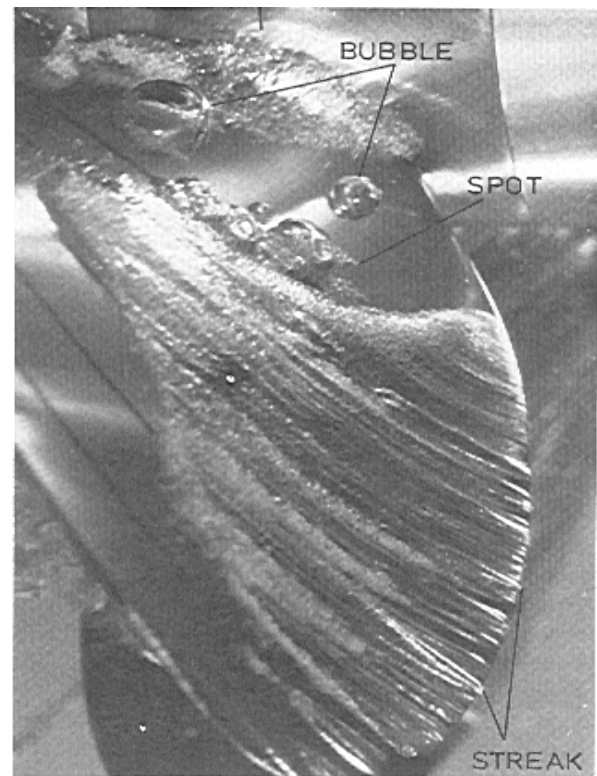
Figure 2 Leading edge, large bubble and root cavitation
