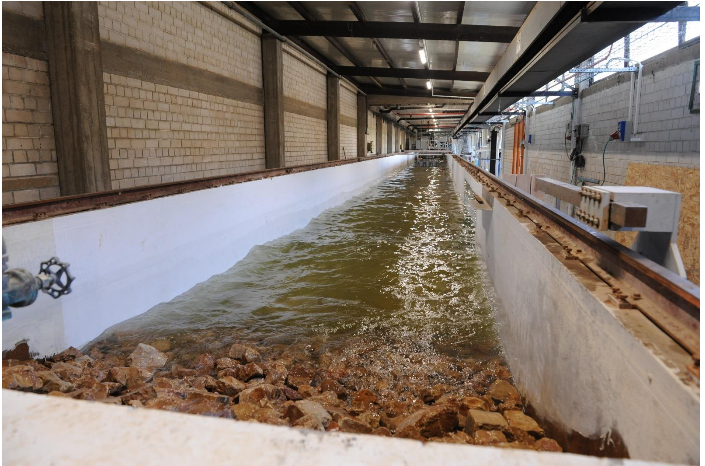
Picture 1: Wave Flume
