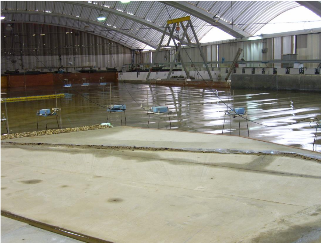
Picture 1: Physical Model Study to Assess Wave Conditions In A Staging Harbor For The Ashdod Port 2015
