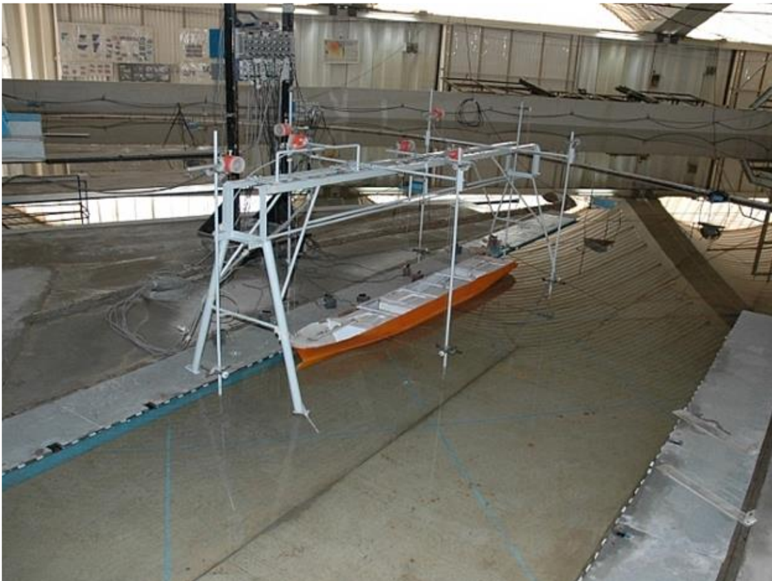
Picture 2: Physical model study to assess mooring conditions of ships along modeled Quay 21 at HAYOVEL, Ashdod
