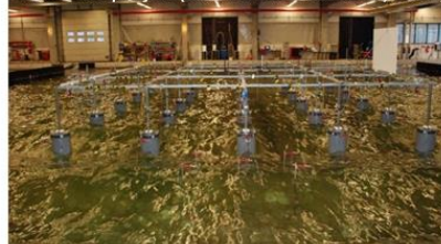
WEC array with 25 heaving buoys from the WECwakes project (taken from Troch et al., 2014)
