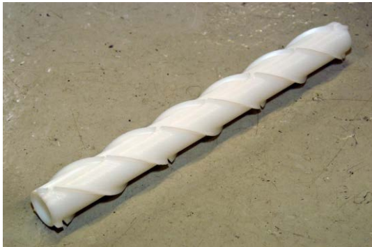
Figure 3 Examples of suppression device models. Upper: strakes (Trim et al., 2005), Lower: fairings (Braaten et al., 2008)
