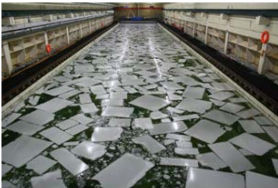
Figure 5: Managed Ice in a model test basin
