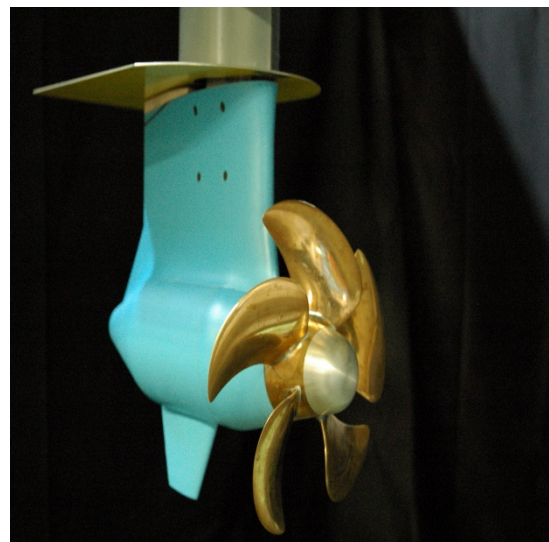
Figure 5 Typical pod unit open water test set-up
