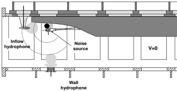
Figure 2: Transfer function measurement set-up in cavitation tunnel
