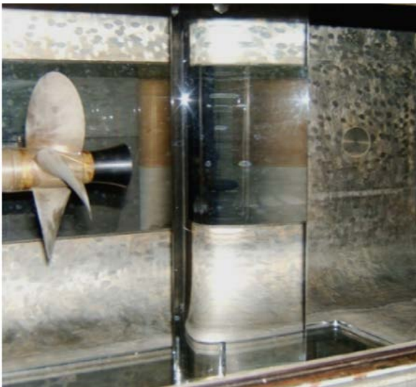
Figure 6. Use of Perspex in order to avoid light reflection (Felli et al., 2011)
