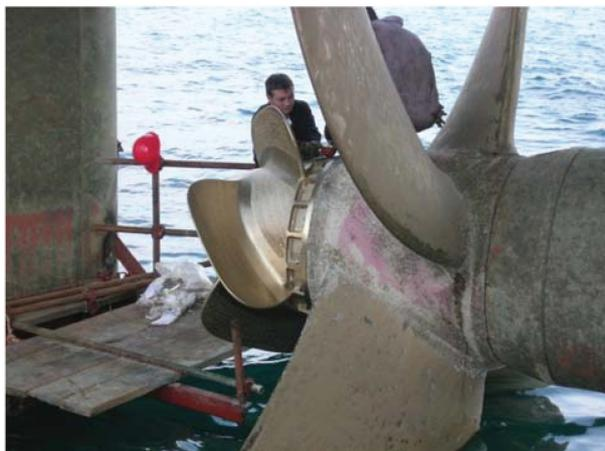
Figure 27 Fitting the PBCF, Hansen et al., 2011
