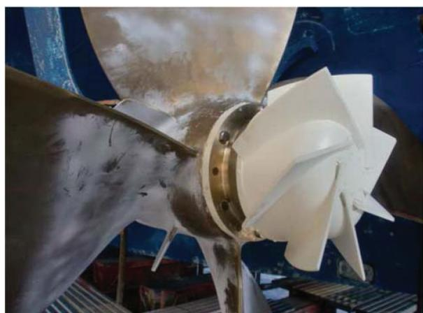
Figure 28 ECO-Cap attached actual ship
