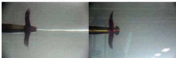
Figure 22 Absorption of hub vortex with DSME cap fin
