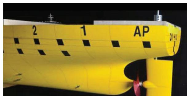
Figure 21 A model ship equipped with SAVER Fin and SARB
