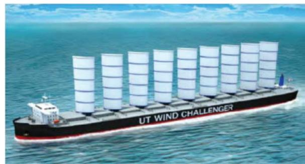
Figure 20 Image of "Wind Challenger" proposed in Ouchi et al. [2013]
