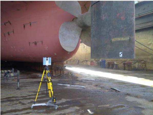
Figure 32 3D laser scanning in a dry-dock, Lloyd's Register, 2016
