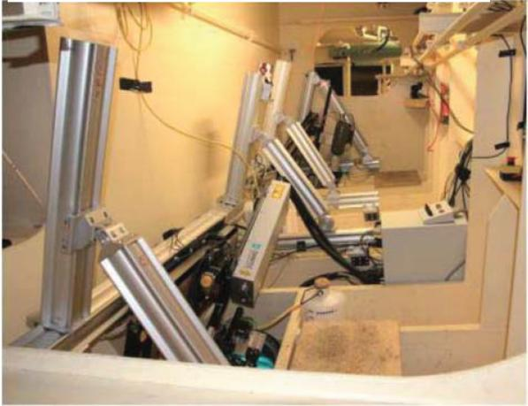
Figure 31 PIV Measurement setup in the steering gear compartment, Kleinwächter et al., 2015
