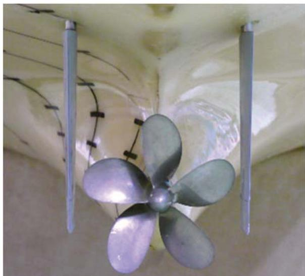
Figure 23 Aft view of a ‘gate rudder’
