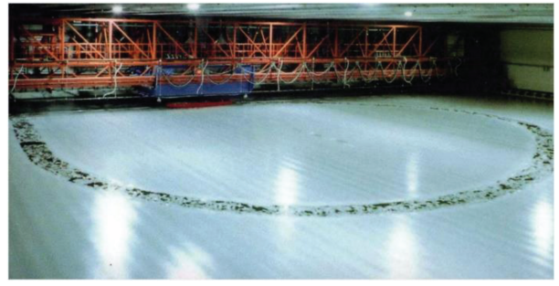
Figure 13 Turning circle test in model scale ice in Aalto Ice Tank.
