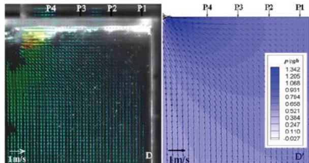
Figure 11 Experimental and numerical velocity field (Yang et al., 2016b)
