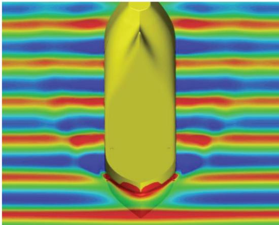
Figure 25 Wave pattern for KVLCC2 advancing in head wave-bow view (Wu et al., 2015 )
