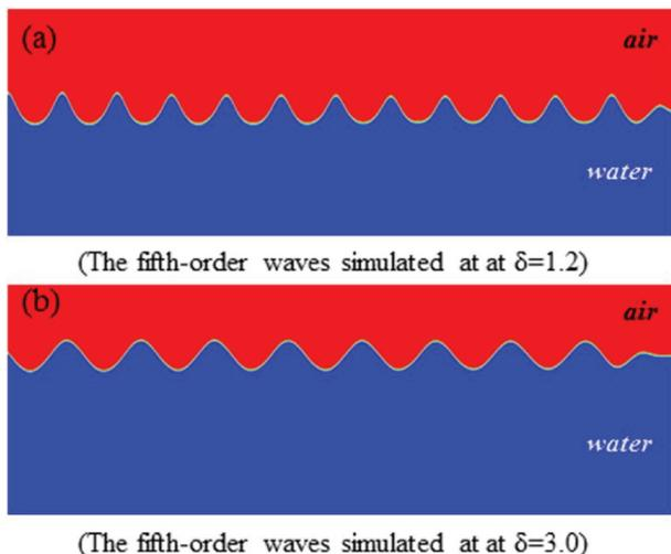
Figure 23 Shallow water waves (Tezdogan et al., 2016)
