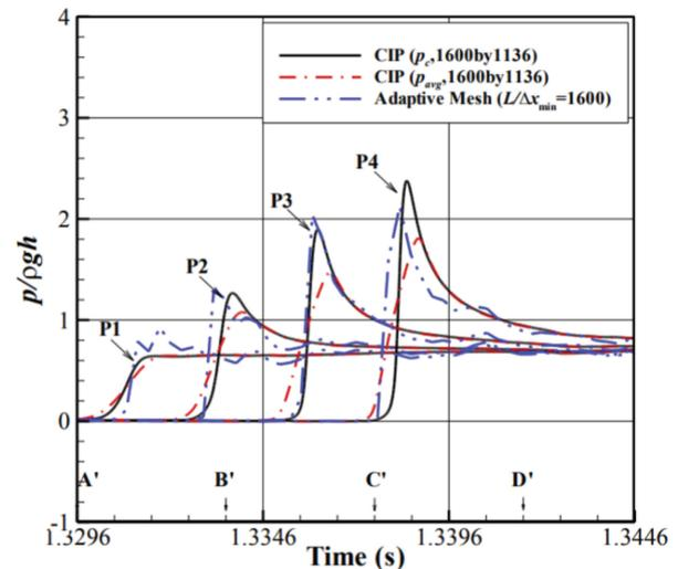
Figure 30 Comparison of pressure time histories with different grid resolution (Yang et al., 2016a)
