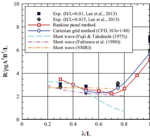
Figure 17 Added resistance: KVLCC2,  $F_n = 0.142$ , heading angle = 180 deg, zoomed on short wave lengths. (Seo et al., 2014)
