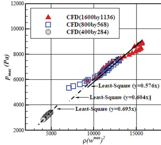
Figure 10 Relationship between peak pressure and square of local maximum vertical velocity (Yang et al., 2016b)
