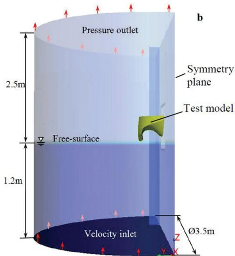
Figure 8 CFD applied to wet deck slamming of a wave piercing catamaran (Swidan et al., 2015)
