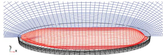
Figure 18 Discretization on free surface in the near field with wet hull and control surface (Pan et al., 2016)
