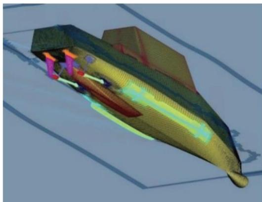
Figure 32 Pressure on CFD grid of ship hull and appendages (Sadat-Hosseini et al., 2015b)
