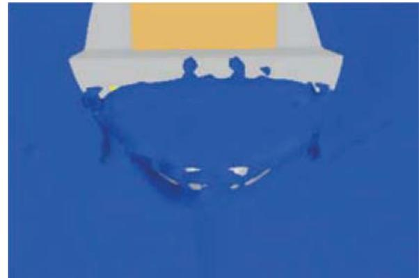
Figure 28 Bow flare slamming and green water (Kim, 2015)
