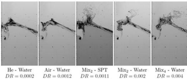
Figure 9 Free surface of the breaking wave before impact with repeated motions and different gas-liquid density ratios (Karimi and Brosset, 2014)
