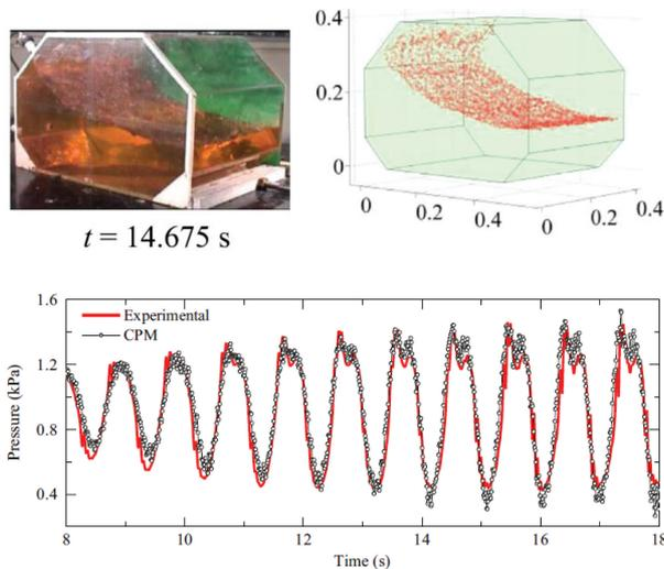
Figure 31 CPM results of sloshing wave in comparison with EFD (Luo et al., 2016)
