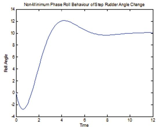
Figure 37 Non-minimum phase zero-the response of a vessel in roll to a hard-over rudder
