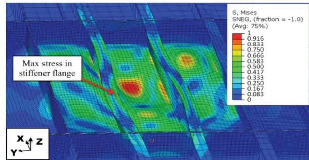
Figure 13 Von Mises stress profile for the stiffener flange corresponding to LC Plate 400 with a load rise time of 3 ms. Scale of deformation:  $\times 20$  (Ringsberg et al., 2016)
