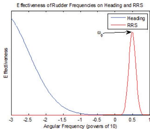
Figure 38 A significant bandwidth separation between heading and roll response (as a function of rudder input)
