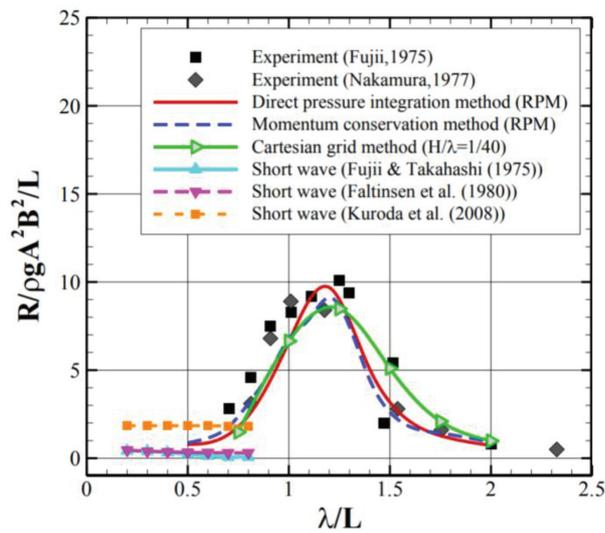
Figure 7 Comparative study on added resistance (Kim Y. et al., 2014)
