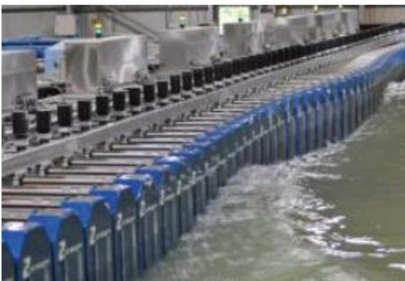
Figure 5 Multi-unit wave generator system
