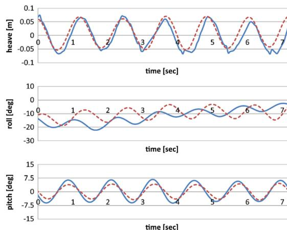
Figure 34 Shipping of green water and ship motions as computed by a SPH method (Kawamura et al., 2016)
