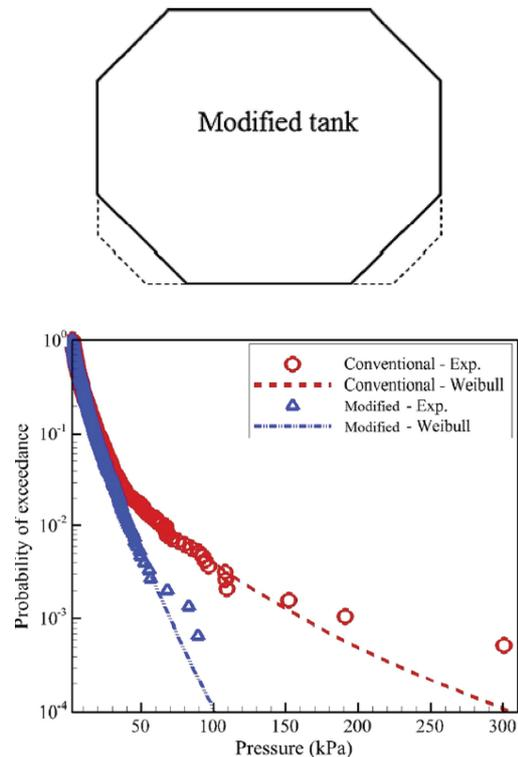
Figure 15 Comparison of sloshing-induced pressures of conventional and modified tanks (Park, J.J. et al. 2015)
