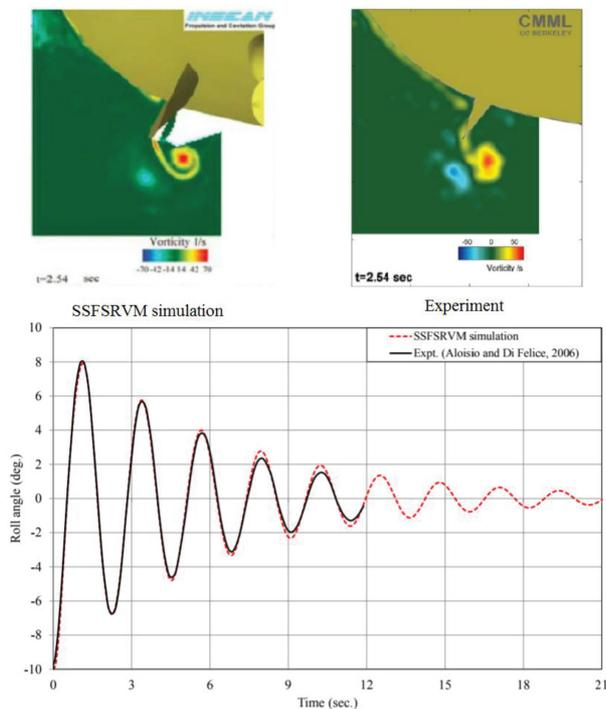
Figure 27 Comparison of CFD and EFD results (Jiang and Yeung, 2016)
