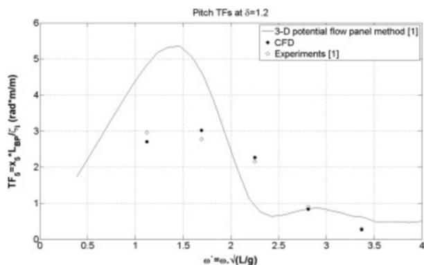
Figure 24 Pitch RAOs using different methods in shallow water (Tezdogan et al., 2016)
