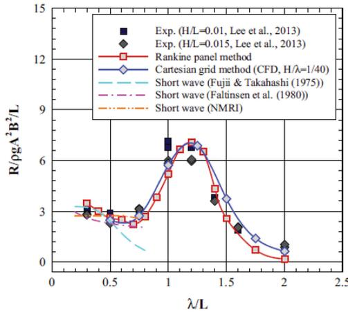
Figure 16 Added resistance: KVLCC2,  $F_n=0.142$ , heading angle = 180 deg. (Seo et al., 2014)
