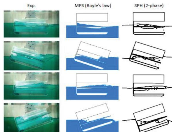
Figure 35 Simulated and experimental free surface comparison inside tank (Le Touzé et al., 2014)
