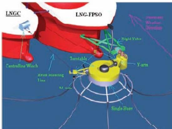
Figure 2.1.4.1 Bow Connection Details of New Concept SPM Mooring System (Zhang et al., 2012)
