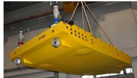
Figure 7.2.3 Ship Model for Thruster-Thruster/Hull Interaction Tests at Samsung Ship Model Basin (Song et al., 2013)
