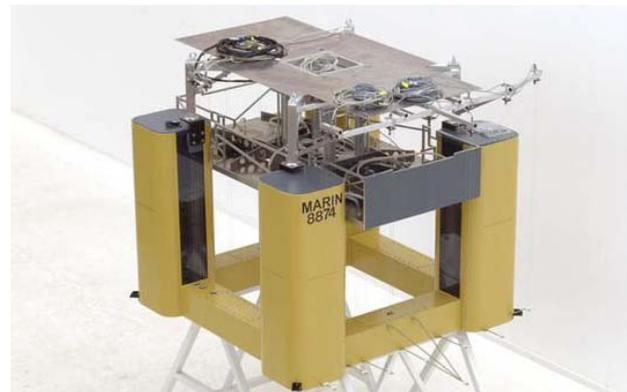
Figure 2.1.2.1 The TLP Model Used in CresT (Hennig et al., 2011)
