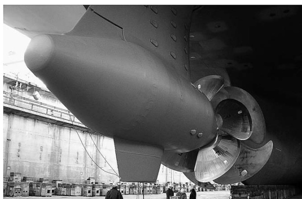
Figure 68: HCRSP mounted on a ROPAX Ferry (Ueda, 2004)
