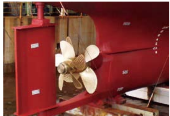
Figure 4: CRP Electric Propulsion system (Hideki, et al. 2011)
