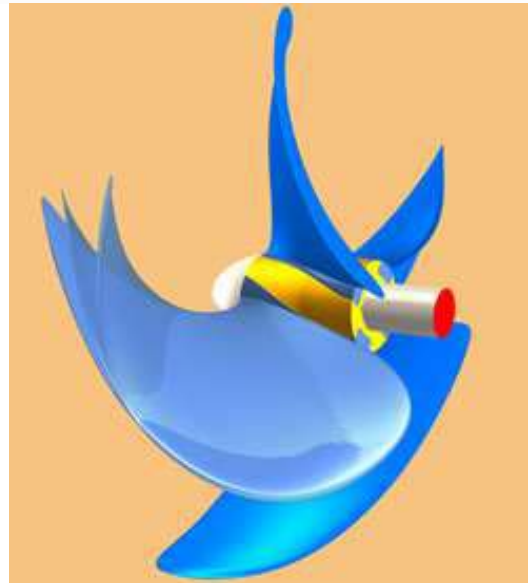
Figure 16: Elastic blade deformation on a composite propeller (Young, 2012).
