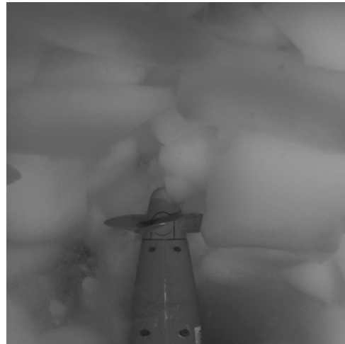
Figure 18: Picture from a high-speed camera of a propeller entering an ice ridge (Brouwer et al. , 2013).
