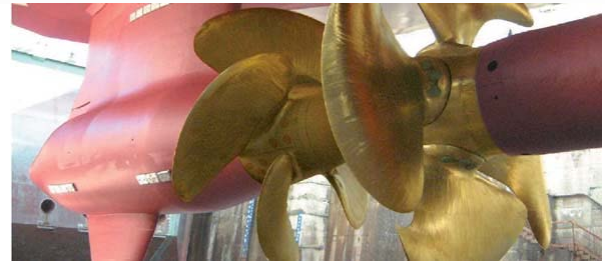
Figure 3: The main propeller (right) with counter rotating, 360 degree azimuthing, ABB Azipod thruster on 200 TEU Container Feeder vessel (Henderson, 2013)
