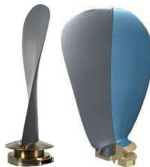
Figure 13: Composite propeller to the RNLN minehunter. (Black, 2011)
