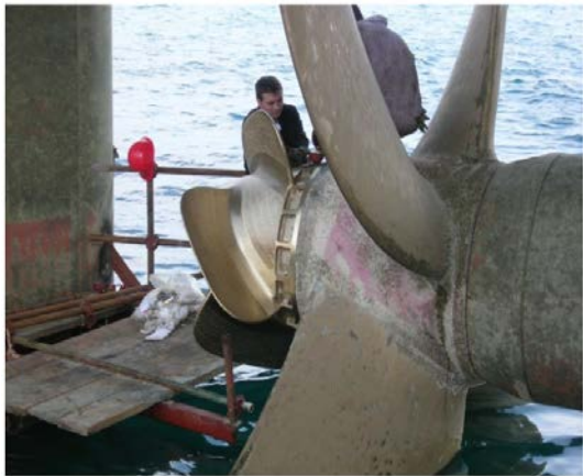
Figure 53: Fitting the PBCF to a full scale ship (Hansen et al. , 2011)
