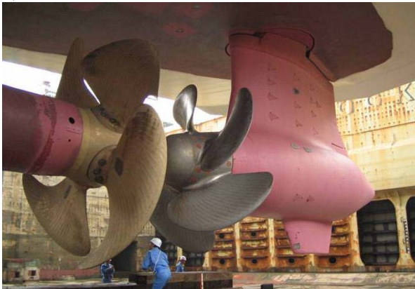
Figure 1: The first ferry with a podded CRP propulsion system (Ueda et al. , 2004)
