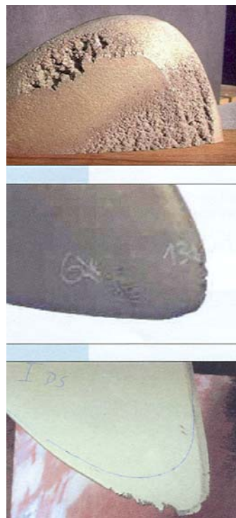
Figure 3.3- Damaged propeller blade tips (Courtesy of HSVA).
