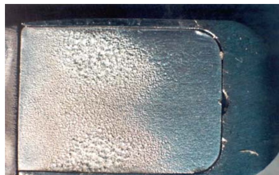
Figure 3.10- Erosion on aluminium sample after 150 minutes (Courtesy of Stinebring)
