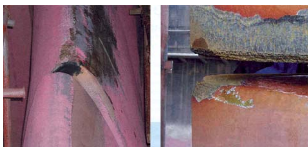
Figure 3.4- Rudder damage (Courtesy of HSVA).
