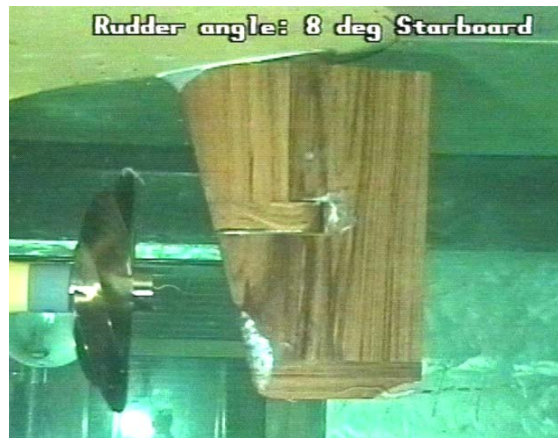
Figure 3.5- Cavitation patterns on a semi-balanced rudder (Courtesy of HSVA).
