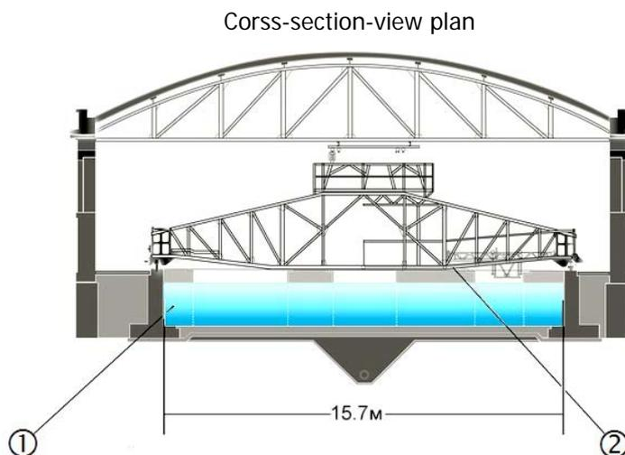
*1 - the basin channel; 2 - manned carriage; 3 - wave generator; 4 - wave absorber; 5 - docks; 6 - sandy bottom simulation.*
