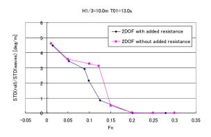
Figure 1 Effect of added resistance on parametric rolling in head waves in the light of numerical simulation in the time domain. (Umeda and Francescutto, 2008)
