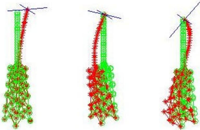
Fig. 3: Support structure modes 1, 3 and 6
