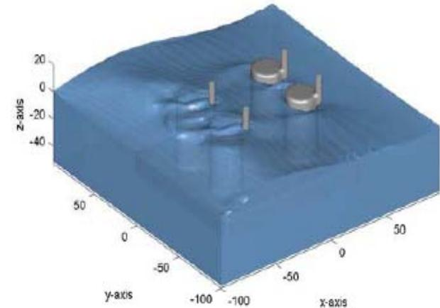
Numerical wave run up calculations
