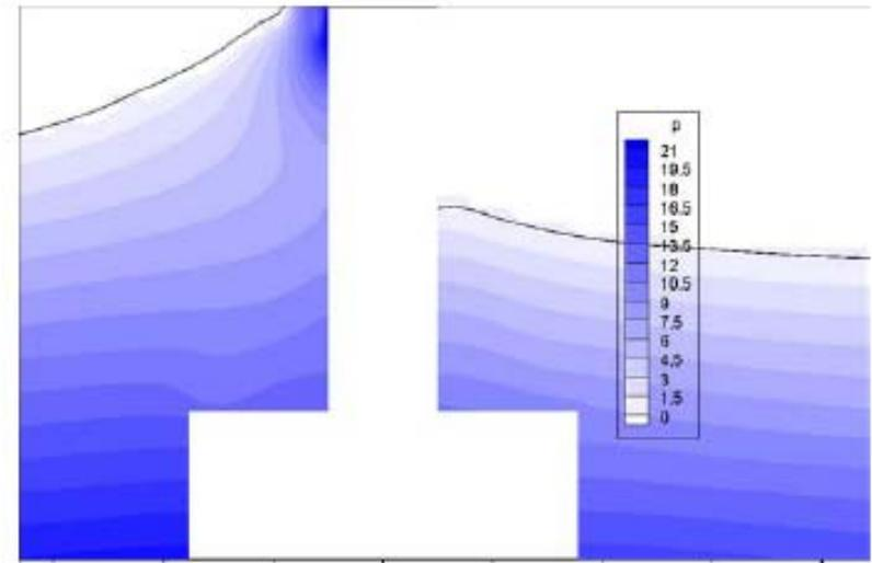
Wave run up and pressure on GBS wind turbine support,
