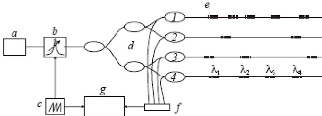
*Fibre optic lines with Fibre Bragg Gratings (FBG)*
