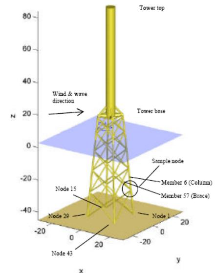
Fig. 2: Support structure model for load analysis
