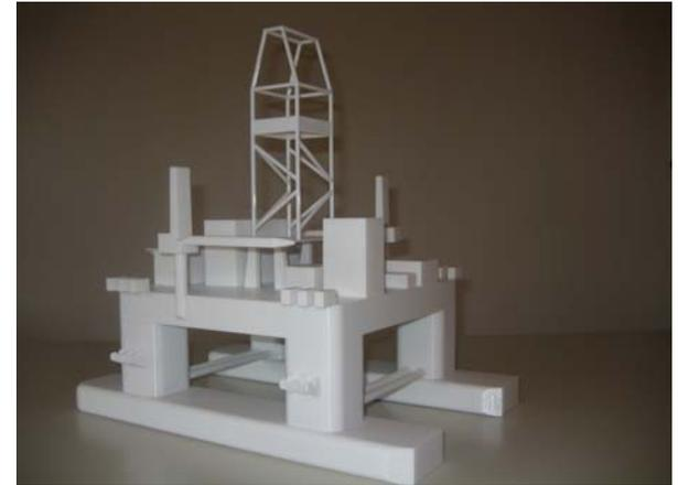
*Scale 1:300 demonstration model of drilling semi, manufactured with rapid prototyping*
