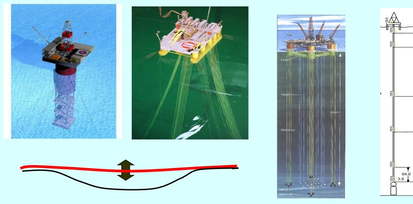
SPAR with D=30 m, U=1.5 m/s,  $f_{St} \cong 0.01$  Hz (T<sub>St</sub>=100 s) Riser with D=0.30 m, U=1.5 m/s,  $f_{St} \cong 1$  Hz
