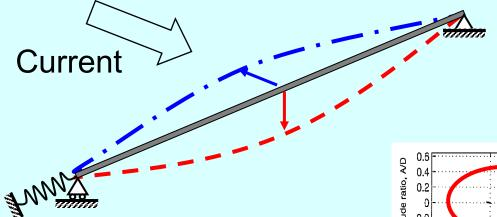
Measured orbits From free spann model tests Small amplitudes, but still more fatigue damage from pure IL than CF in many cases
