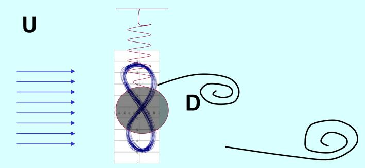
Shedding frequency (fixed cylinder)  $f_{st} = St U/D$ ,  $St \approx 0.15 - 0.3$
