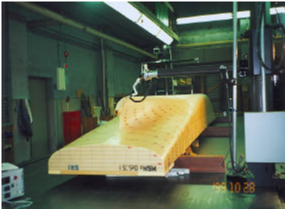
(a) Model Inspection Table and 3-D Digitizer
