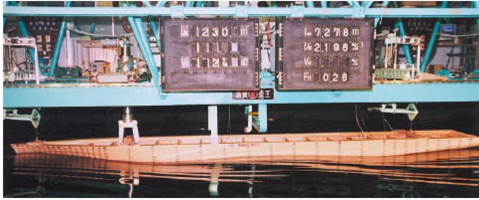
Fig. 7 Resistance Test on NMRI M.S. No. 631 at NMRI 400m Towing Tank
