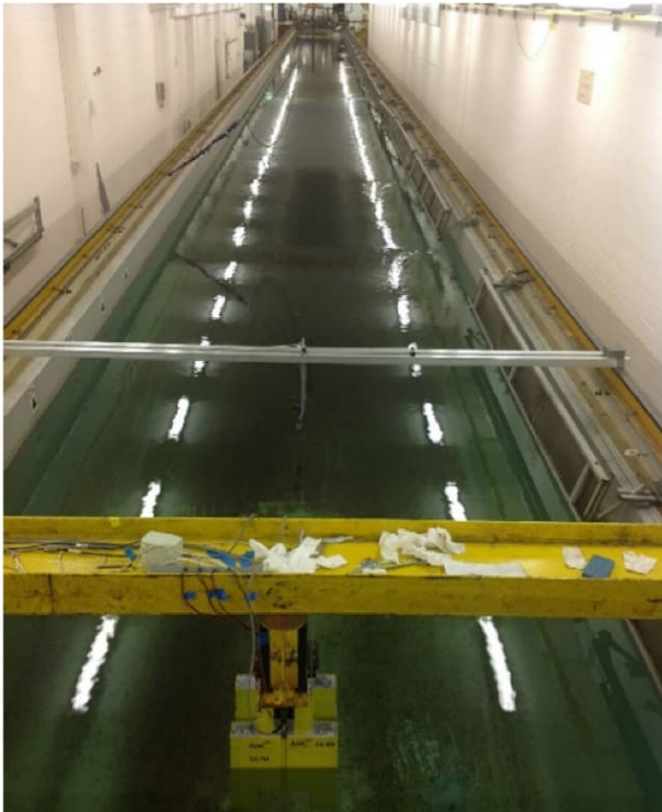
Figure 5: A general view of the AMC towing tank showing the OWC model installed in the tank, looking towards the beach. (Elhanafi et al. 2017)
