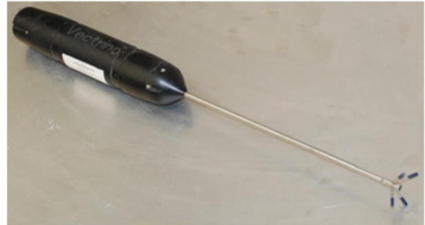
Figure 1: Example of Acoustic Doppler Velocimeter (from Shan et al. (2010))
