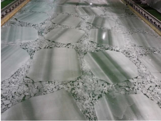
Figure 11: managed ice field in the model basin (60 m long and 12 m wide basin as an example, Wang et al., 2016)
