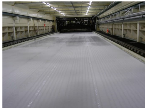
Figure 1: Ice sheet cut free at the sides
