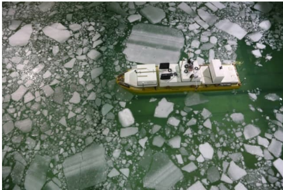
Figure 12: A mixture of floe size in the model basin (Wang et al., 2016)
