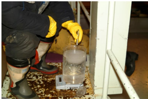
Figure 9: Force balance measurement without displacement recording (Option C).
