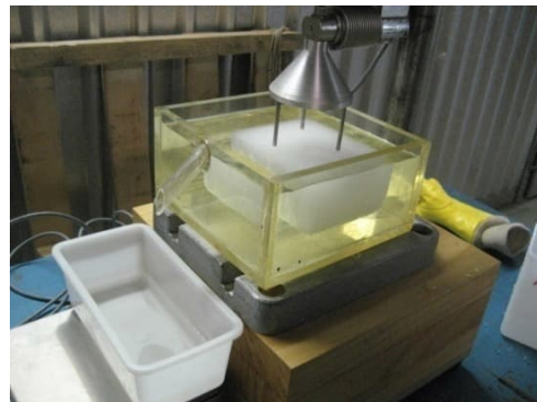
Figure 7: Ex-situ density measurement setup (Option A).
