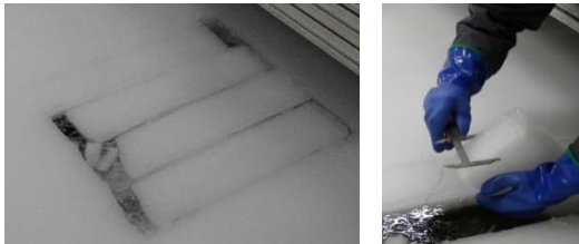
Figure 16: Ice thickness measurements with calliper.
