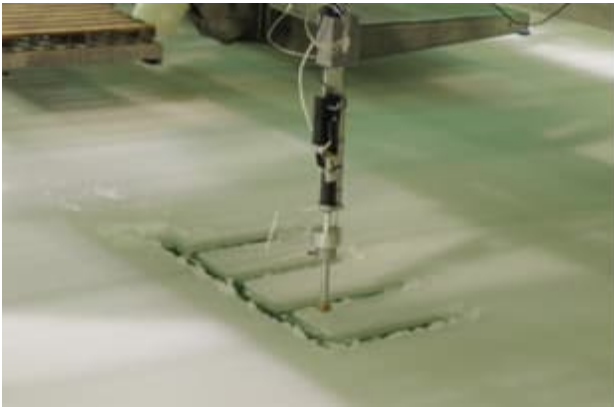
Figure 2: Setup of in-situ cantilever beam test.
