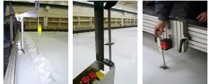
Figure 17: Ridge-profiling device to determine keel depth and sail height.
