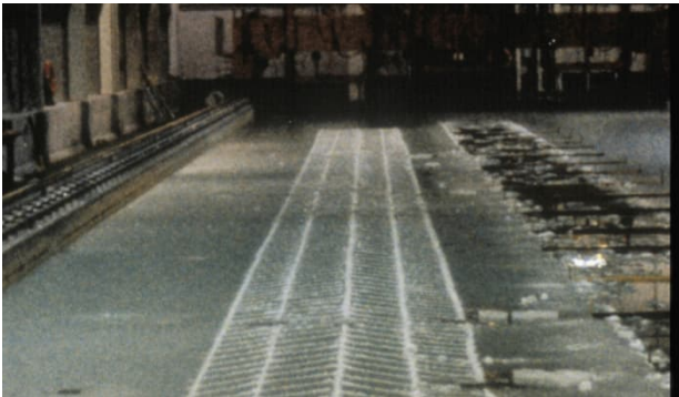
Figure 3: Cutting pattern of pre-sawn ice
