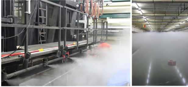
Figure 1: Water is sprayed under high pressure into the air of the pre-cooled ice tank forming crystal nuclides which settle down on the water surface
