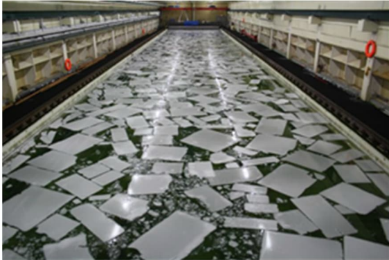
Figure 5: Managed Ice in a model test basin
