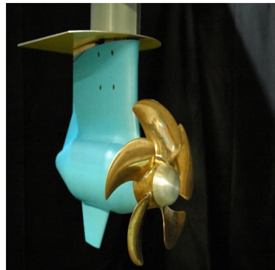
Figure 5 Picture of pod unit open water test set-up
