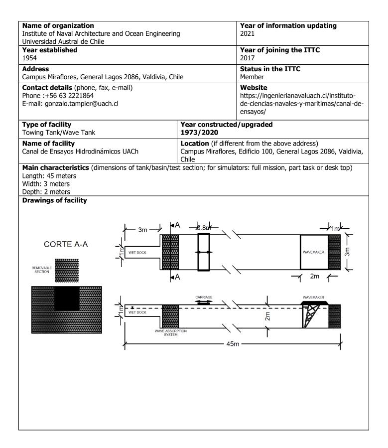
**Detailed characteristics** (carriages, wave/current/wind generators, instrumentations, etc.) **Carriage:** Unmanned aluminum structure mounted on linear bearings, driven by a 5 kW power servomotor. Maximum carriage speed: 5 m/s
