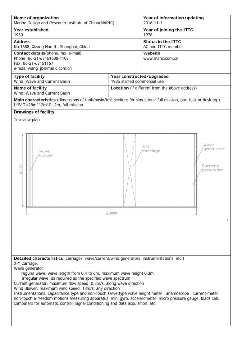
**Applications**(Tests performed) Wind, wave and current test of ships and ocean structures; force and motion measurements for ships and floating offshore structures in different sea conditions, force measurements for fixed offshore structures.
