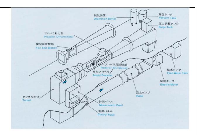
**Detailed characteristics** (carriages, wave/current/wind generators, instrumentations, etc.) **Propeller Test Section**
