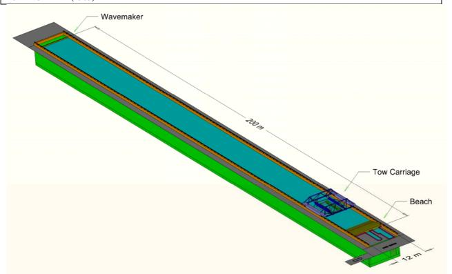
**TOWING CARRIAGE**: Single manned carriage with 8 wheel synchronous motor drive, 85,000 kg, 746 Kw power, 0.001 m/s – 10 m/s speed range. Test frame adjustable for model size.
