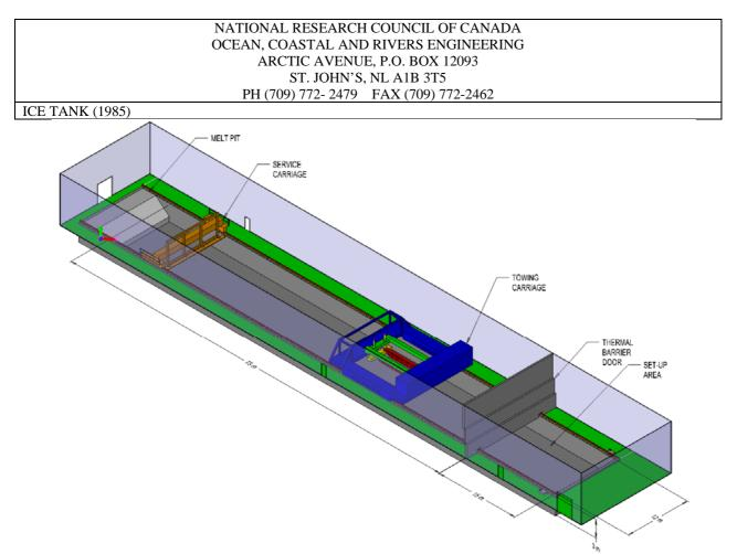
**TOWING CARRIAGE**: Manned carriage with a 4 wheel or rack synchronous motor drive, test frame adjustable for model size, 80,000 kg mass, 745 kW of power for a drive force of 60 kN, speed range 0.0002 m/s to 4.0 m/s. Also includes and underwater Frame 9.4m long by 6.3 wide running on pneumatic wheels over the bottom of the tank, connected to tow carriage. Capable of speeds of up to 1.0m/s.
