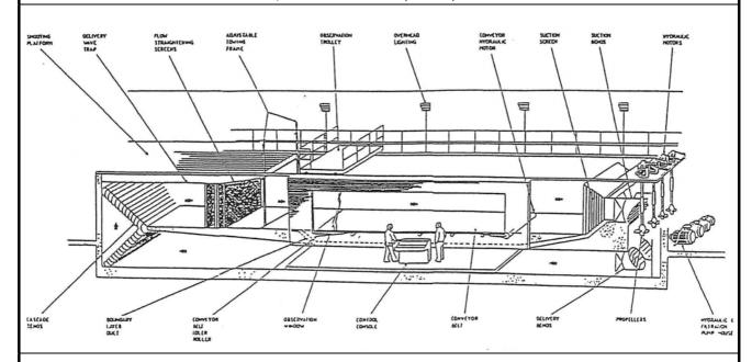
WORKING SECTION: length 17.2m, width 5.0m, depth 2.4m
