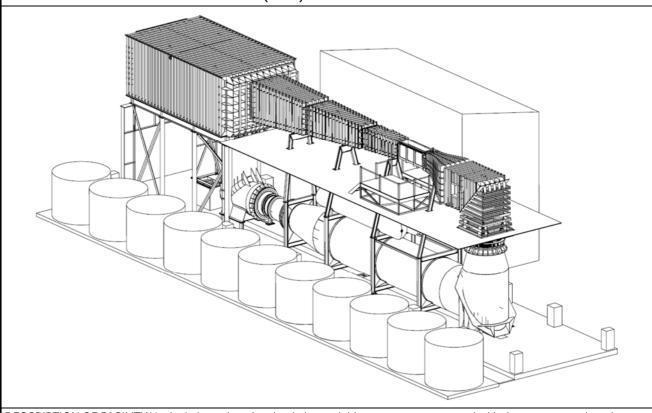
**DESCRIPTION OF FACILITY:**Vertical plane,closed recirculating variable pressure water tunnel with downstream tank and resorber, test section dimensions 0.6 x 0.6 x 2.6m long, contraction ratio 7.12:1, circuit volume 365 cubic metres, low background noise and vibration levels, rapid degasser, online nuclei and incondensable gas injection and separation, working section ceiling boundary layer thickness control.
