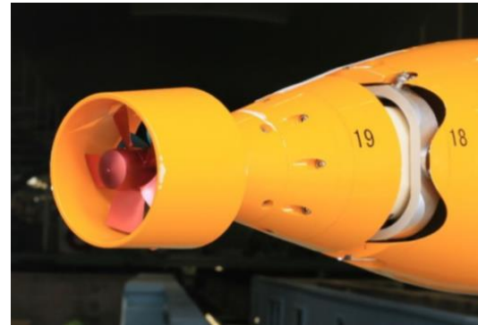
Figure 109. VTS integrated with the NSRC free running model (Maki et al., 2018)
