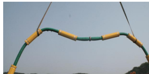
Figure 267: Flexible hoses with buoyancy materials (Yoon et al., 2011)
