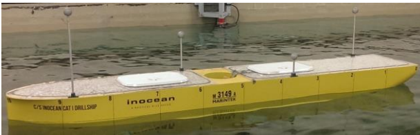
Figure 160: The model test for thruster-assisted position mooring (Bjørnø et al., 2017)
