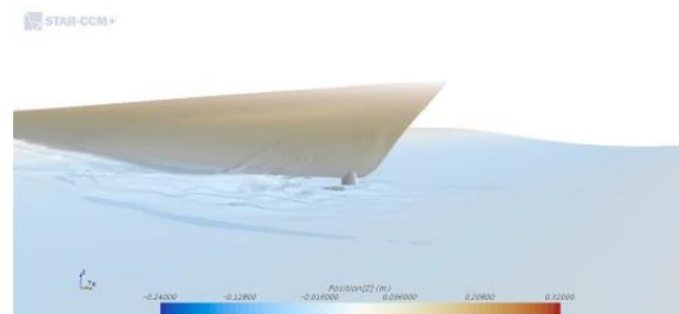
Figure 315: Snapshot of the instant where the T-foil enters the water (Li et al, 2020).
