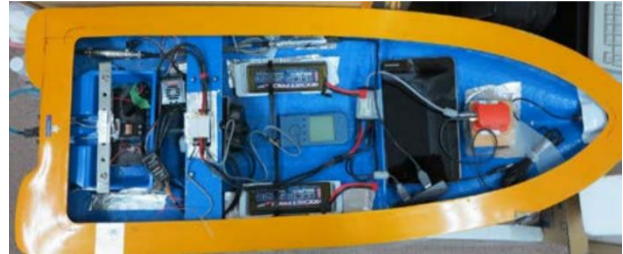
Figure 341: Instrumentation of free running HSMV model (Katayama et al., 2014)
