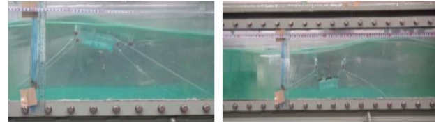
Figure 194: Controllable depth cage model test when the cage was at water surface (left) and at the submerged depth (right) (Yu et al., 2018)
