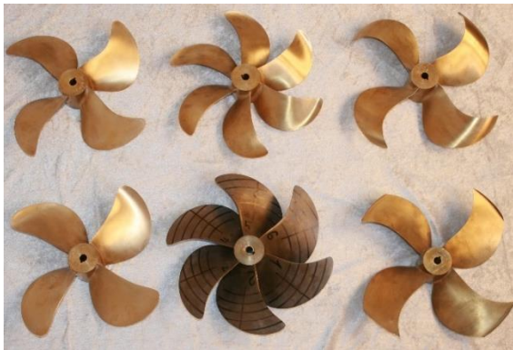
Figure 66: Original (dark) and the five new (shiny) model propellers
