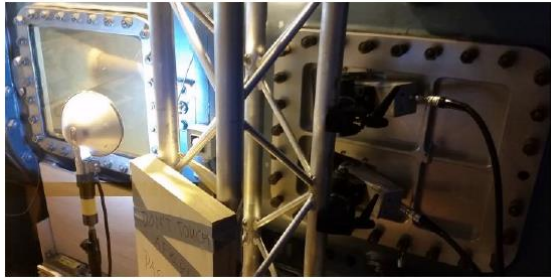
Figure 1: Camera setup in the cavitation tunnel (Grasso et al., 2019)
