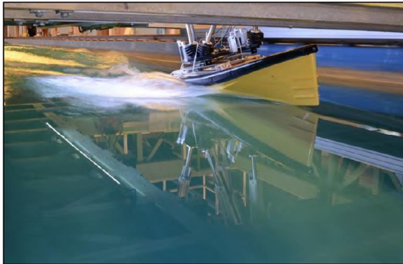
Figure 77: Model test run in heeled condition (Bonci et al., 2017)
