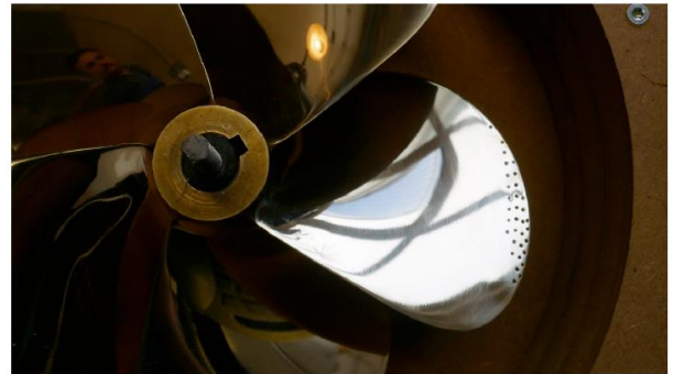
Figure 7: PressurePores™ as applied on the Princess Royal propeller (Aktas et al., 2019)
