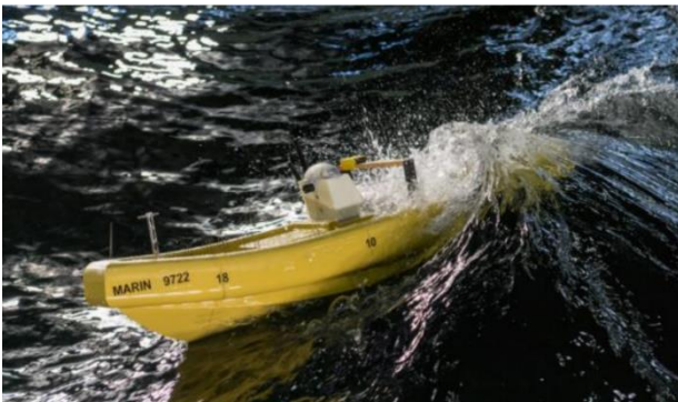
Figure 319: Fully free running RHIB model during seakeeping model tests (Van Walree and Thomas, 2017)
