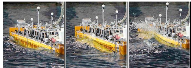
Figure 135: Evolution of a beam sea extreme green water event during model tests (Silva et al., 2017a)
