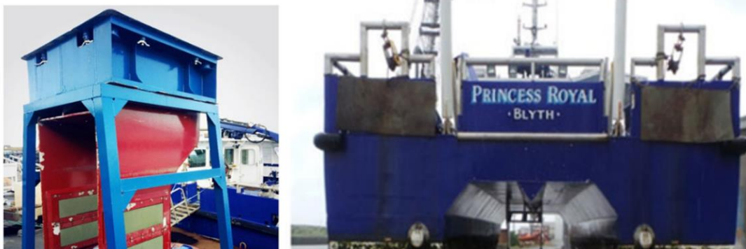
Figure 33: Testing panels installed on the twin strut assembly (left) and the strut system deployed under the moon-pool plug (right) (Yeginbayeva and Atlar, 2018)
