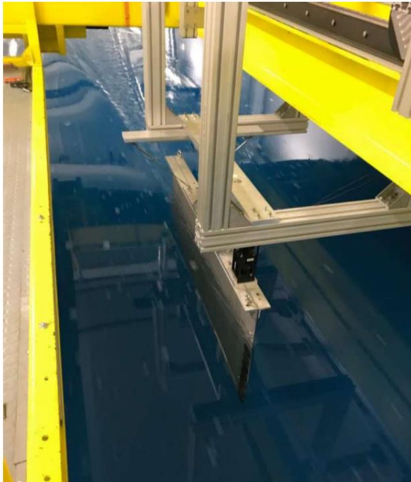
Figure 20: Flat plate towed at 4.5 m/s (Ravenna et al., 2019)
