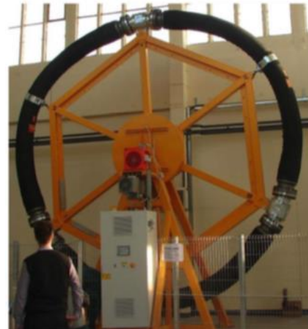
Figure 277: Rotating full-scale abrasion tester (Neale et al., 2017)
