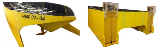
Figure 327: Wavepiercing catamaran model fitted with RCS (AlaviMehr et al., 2019)
