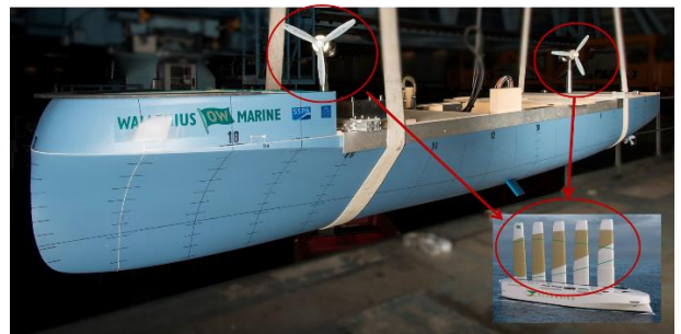
Figure 285: Simulation of sail forces via rpm azimuth-controlled fans, from Gerhardt and Santén (2021)
