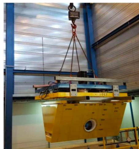
Figure 8: Experimental setup to measure performance of rim driven tunnel thruster (Klinkenberg et al., 2017)
