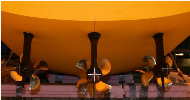
Figure 44. Model scale triple pod installation
