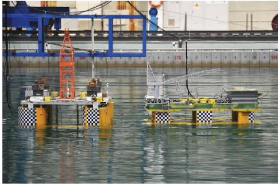
Figure 150: Experiment of TLP-TAD coupled system (Dong et al., 2019)
