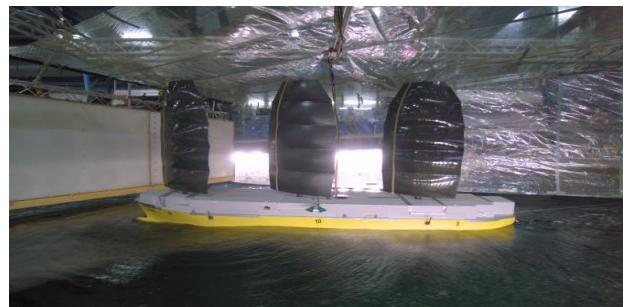
Figure 284: “Wind tunnel” in MARIN’s seakeeping basin, from Eggers and Kisjes (2019)
