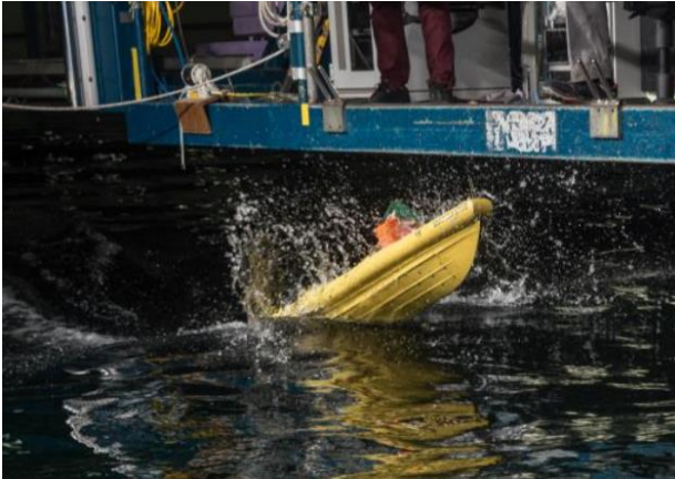
Figure 342: Fully free running model of the FRISC RHIB (Van Walree and Struijk, 2021)
