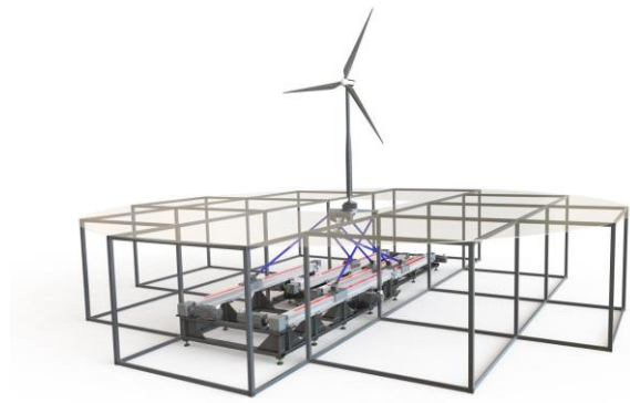
Figure 209: 6-DoF Robotic platform “HexaFloat” for wind tunnel tests (Bayati et al., 2014)
