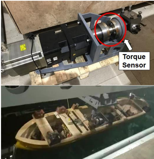
Figure 367: Forced roll mechanism developed by MARIC
