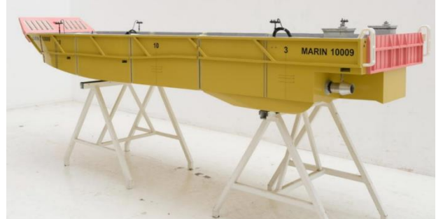
Figure 320: Captive model tests with a SAR boat of the Royal Netherlands Sea Rescue Institution (Bonci et al., 2017b)
