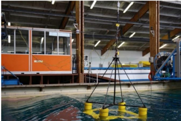
Figure 221: Scale model during wave tank tests (Matoug et al., 2020)
