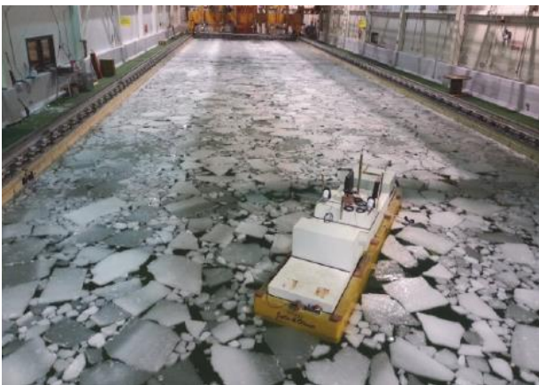
Figure 158: View of the ice basin and the model DP vessel (Sayed et al., 2017)
