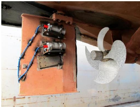
Figure 3: Stereo camera setup installed on the port side of the diving support vessel "Nautilus" (Grasso et al., 2019)
