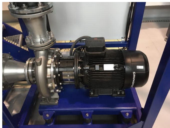
Figure 5: Centrifugal pump circulating the flow in the flume.
