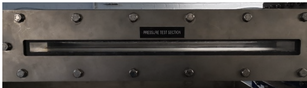
Figure 3: Test section equipped with a Perspex side window.
